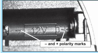
FIG. 8-2 Match battery polarity.
